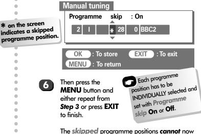
The **skipped** programme positions **cannot** now be selected by the  $P \triangleq (\frown)$  and  $P \bigtriangledown (\bigcirc)$  buttons or by the controls on the front of the TV, but can still be accessed by the number buttons on the remote control. To turn **Programme skip OFF**, repeat the procedure on the chosen channel.
